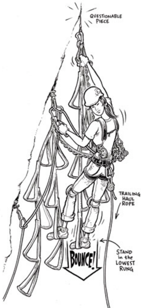
Figure 1: A climber bounce-testing while leading an aid pitch. Note the aider and daisy setup. If her top pieces passes the test, she'll move up into the higher set of aiders and clip the low ones to her harness gear loop. It's possible that the bounce-test will rip out the piece. If so, she'll catch herself on the lower aiders and try another placement. Illustration by Mike Clelland
